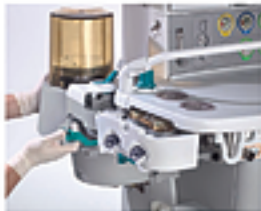
One switch and no tools disengage the setting system facilitates easier cleaning and reduced maintenance time
